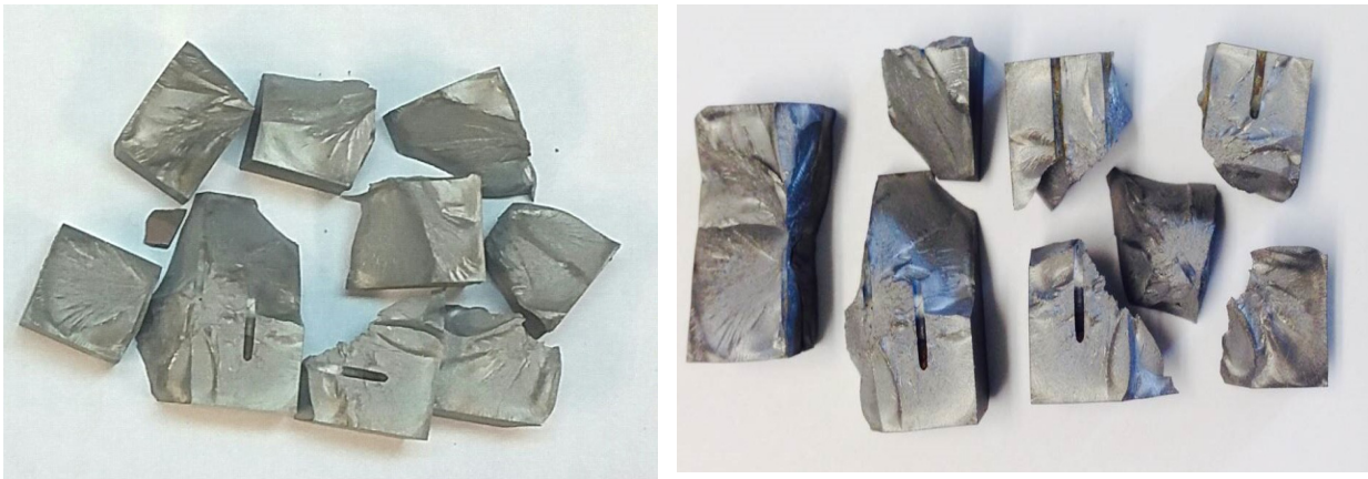
Figure 4.—(a) Fractured remains after thermal treatment using immersion method. (b) Fractured remains after thermal treatment using agitation method.
