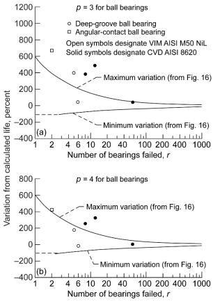
Figure 22.—Effect of VIM–VAR M50 NiL and CVD AISI 8620 steels and load-life exponent on bearing life (Ref. 90). (a) Load-life exponent *p* is 3 for ball bearings (from Fig. 18). (b) Load-life exponent *p* is 4 for ball bearings.
