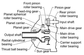
Figure 24.—Commercial turboprop gearbox (Ref. 94).
