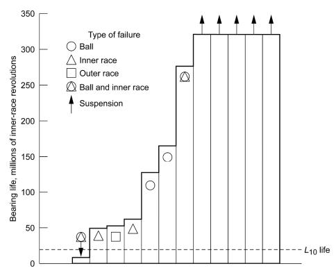
Figure 9.—Rolling-element fatigue lives of AISI 52100 204-size angular-contact ball bearings. Contact angle is 10°; outer-race temperature, 79 °C (175 °F); thrust load, 1108 N (249 lb); inner-ring speed, 10 000 rpm; lubricant, MIL–L–7808; *L*<sub>10</sub> life, 20.5×10<sup>6</sup> inner-ring revolutions (34.2 hr); and failure index, 7 out of 12 (Ref. 44).
