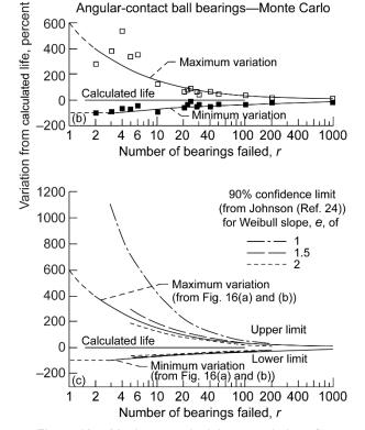
Figure 16.—Maximum and minimum variation of  $L_{10}$  lives as percent of calculated  $L_{10}$  for groups of r bearings and 90% confidence limits based on Weibull slope and number of bearings failed r (Ref. 90). (a) 50-mm-bore deep-groove ball bearing. (b) 50-mm-bore angular-contact ball bearing. (c) 90% confidence limits.
