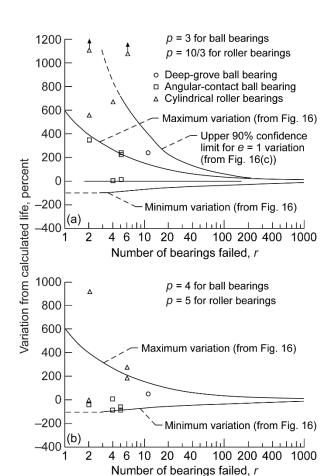
Figure 20.—Effect of VAR AISI M–50 steel and load-life exponent on bearing life (Ref. 90). (a) Load-life exponent *p* is 3 for ball bearings and 10/3 for cylindrical roller bearings (from Fig. 18). (b) Load-life exponent *p* is 4 for ball bearings and 5 for cylindrical roller bearings.
