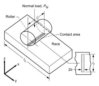
Figure 4.—Roller-race model for line contact.
