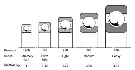
Figure 10.—Effect of bearing series on relative sizes and dynamic capacities,  $C_D$ , of 40-mm-bore deep-groove ball bearings (Ref. 31).
