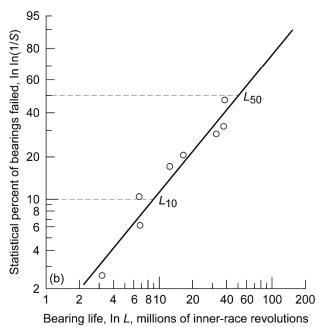
Figure 1.—Weibull plot where (Weibull) slope of tangent of line is e; probability of survival  $S_{\beta}$  is 36.8 percent at which  $L = L_{\beta}$ , or  $L/L_{\beta} = 1$ . (a) Schematic where S is probability of survival. (b) Rolling-element bearing fatigue data where InIn (1/S) is presented in ordinate as statistical percent of bearings failed.
