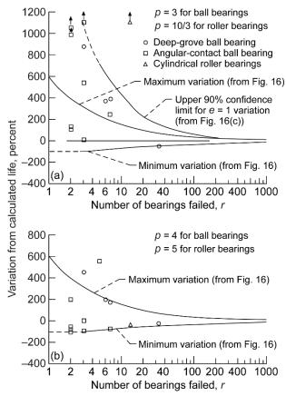
Figure 21.—Effect of VIM–VAR AISI M–50 steel and load-life exponent on bearing life (Ref.90). (a) Load-life exponent *p* is 3 for ball bearings and 10/3 for cylindrical roller bearings (from Fig. 18). (b) Load-life exponent *p* is 4 for ball bearings and 5 for cylindrical roller bearings.
