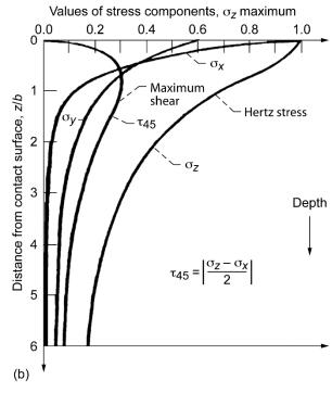
Figure 5.—Subsurface stress field under line contact.
