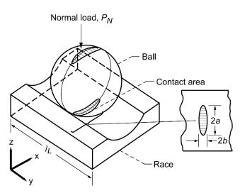
Figure 3.—Ball-race model for point contact.
