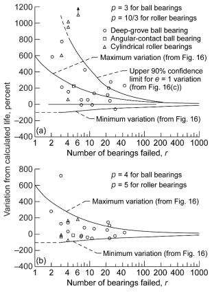
Figure 19.—Effect of CVD AISI 52100 steel and load-life exponent on bearing life (Ref. 90). (a) Load-life exponent p is 3 for ball bearings and 10/3 for cylindrical roller bearings (from Fig. 18). (b) Load-life exponent p is 4 for ball bearings and 5 for cylindrical roller bearings.
