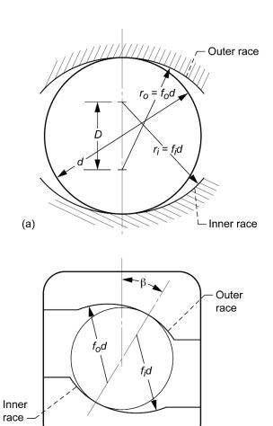
Figure 7.—Ball-race conformity. (a) Deep-groove ball bearing. (b) Angular-contact ball bearing.
