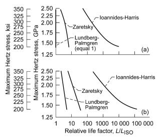
Figure 15.—Comparison of life models for rolling-element bearings with ANSI/ABMA and ISO standard without a fatigue limit. Fatigue-limiting shear stress for  $\tau_{45}$  assumed for loannides-Harris model, 276 MPa (40 ksi) (Ref. 85). (a) Ball bearings. (b) Cylindrical roller bearings.
