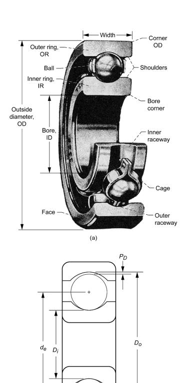
Figure 6.—Deep-groove ball bearing. (a) Schematic. (b) Cross section without cage.
