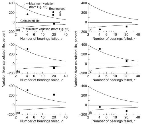
Figure 17.—Rules for comparing bearing life results to calculated life (Ref. 90).
