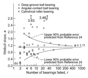
Figure 23.—Variation of Weibull slope *e* compared with predicted 90% probable error. (a) Extremes of Weibull slope from Monte Carlo testing for each group of 10 bearing trials of *r* bearings (data from Ref. 90). (b) Weibull slopes from 51 sets of ball and roller bearings (data from Refs. 91 and 92).
