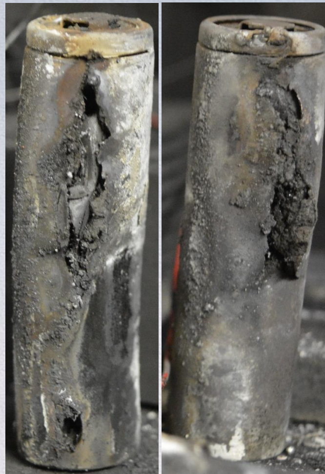
ISC device in 3 rd wind
