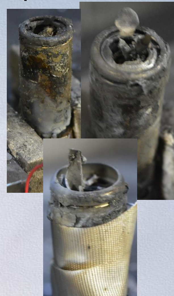
Circumferential heater near bottom of can wall
