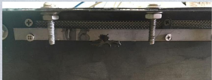
Mesh 40 & 30 steel screens arrest flames and sparks
