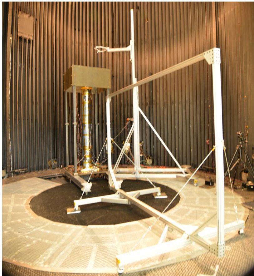
Figure 16. MRTS mounted 2m off-center in Space Simulator.
