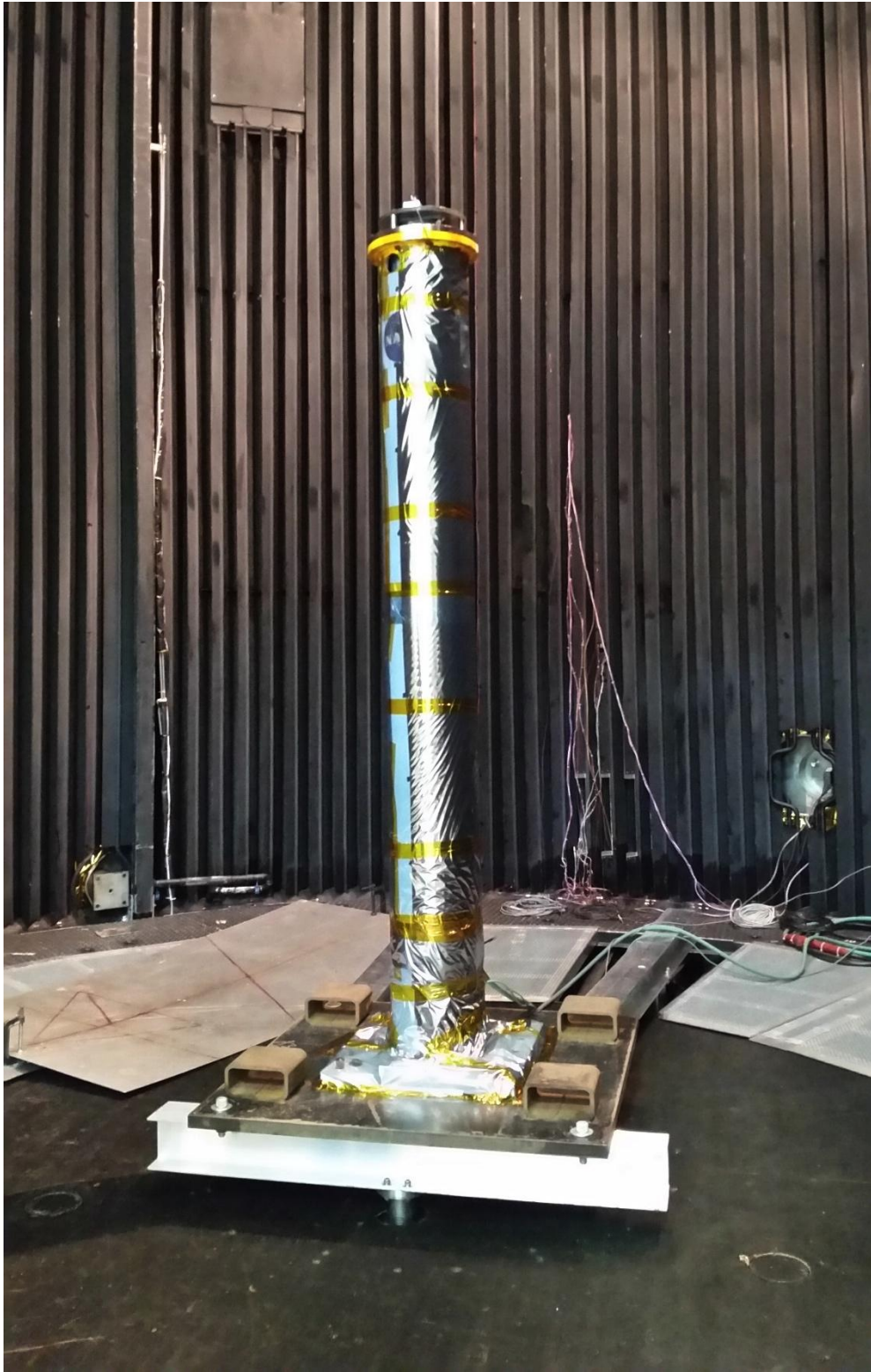
Figure 13. MRTS assembly sans blast shield in Space Simulator.
