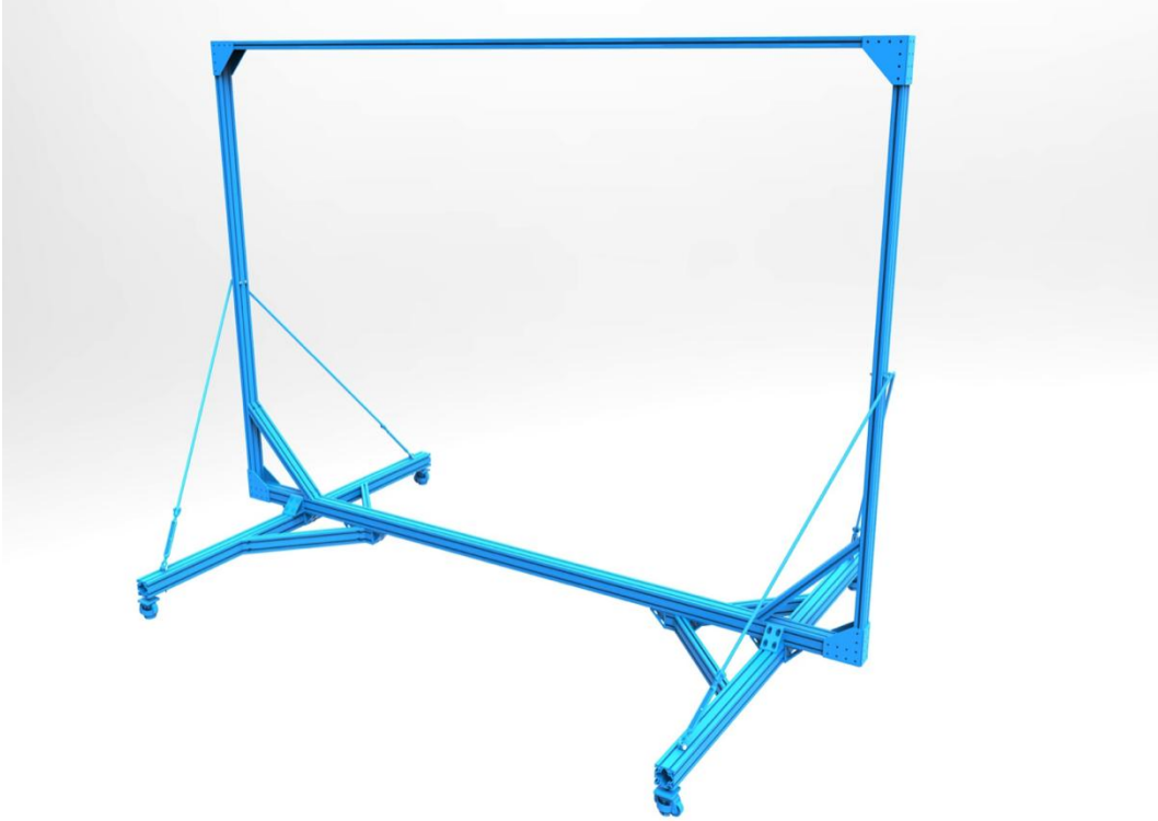
Figure 8. Tuft frame (without tufts).
