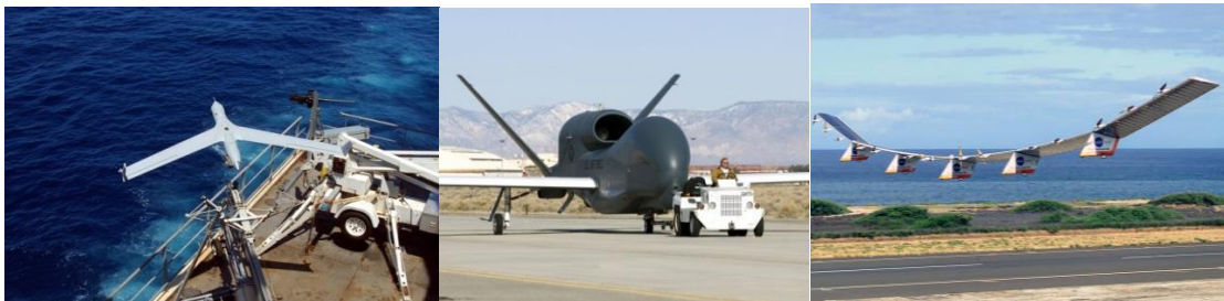
Figure 1. Three examples of remotely piloted aircraft. (1) The 18 kg, catapult-launched Insitu ScanEagle; (2) 6,700 kg High Altitude Long Endurance (HALE) Global Hawk; (3) AeroVironment Helios Prototype, a solar powered flying wing designed for long-duration, high-altitude missions in the stratosphere.
