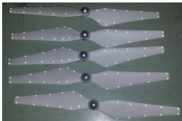
Figure 8: The 5 tested DJI Phantom 3 blades with illuminated targets. Some targets fell off during the higher RPM measurements.
