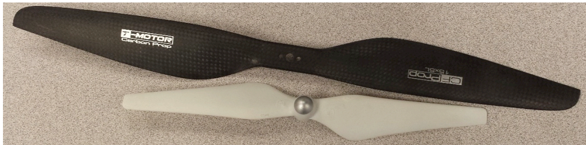
Figure 2: The two types of commercially available quadcopter blades that were studied. The top one is the carbon fiber T-motor 15x5 blade while the bottom one is the DJI Phantom 3 blade.
