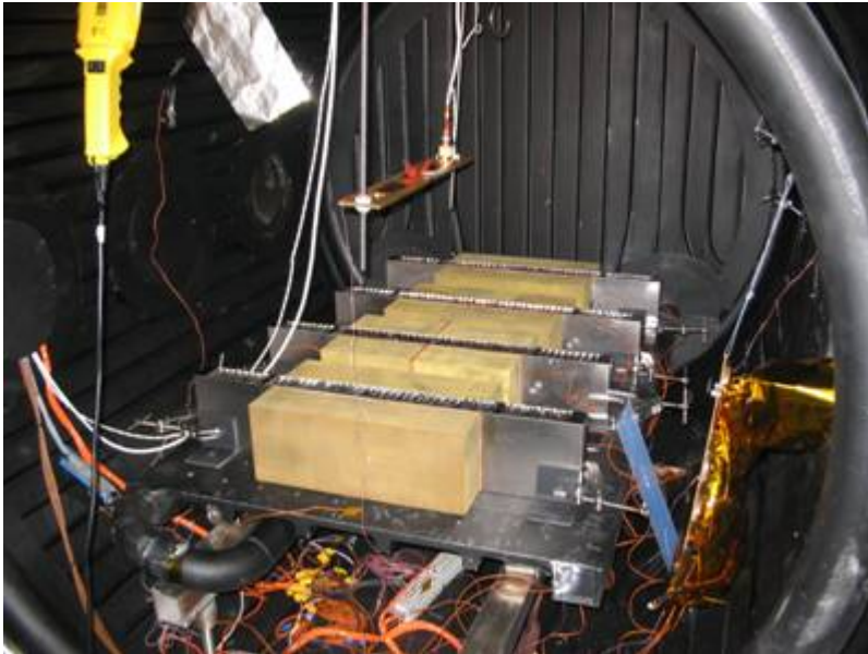
Modal Testing of Bend Coupons
