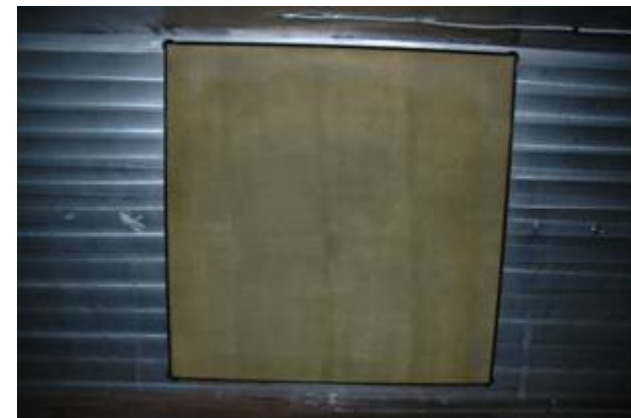
Acoustic Panel installed in TAFA Exposed Side (Flow is left-to-right)
