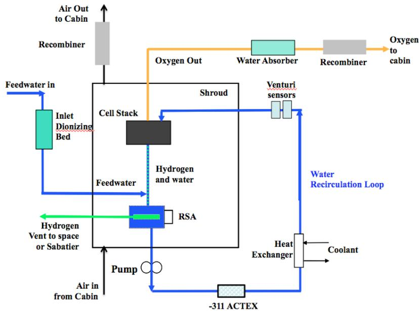
Figure 4. Proposed schematic of a future OGA. (Takada et al., 2015-115)
