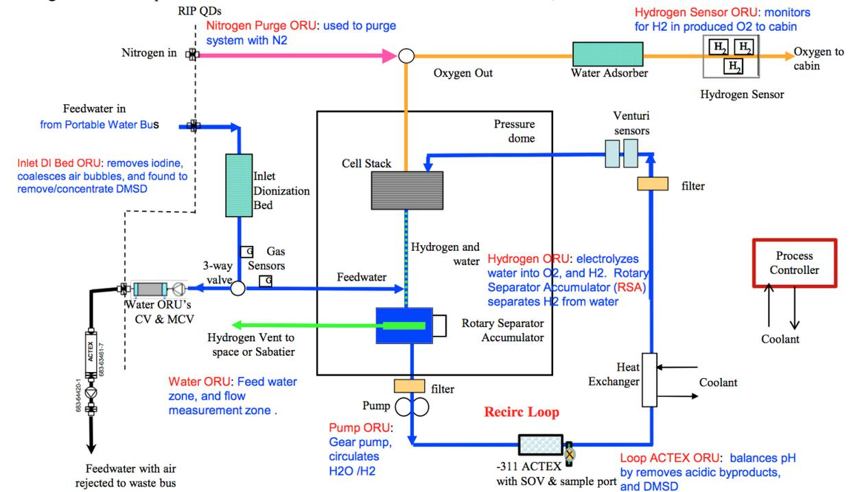
Figure 1. Simplified OGA schematic. (Takada et al., 2015-115)
