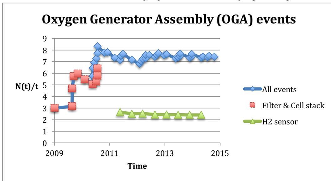
Figure 2. The time averaged cumulative failure and maintenance rate,  $N(t)/t$ , for all the events, for the combined Filter and Cell stack group, and for the H2 sensor group.
