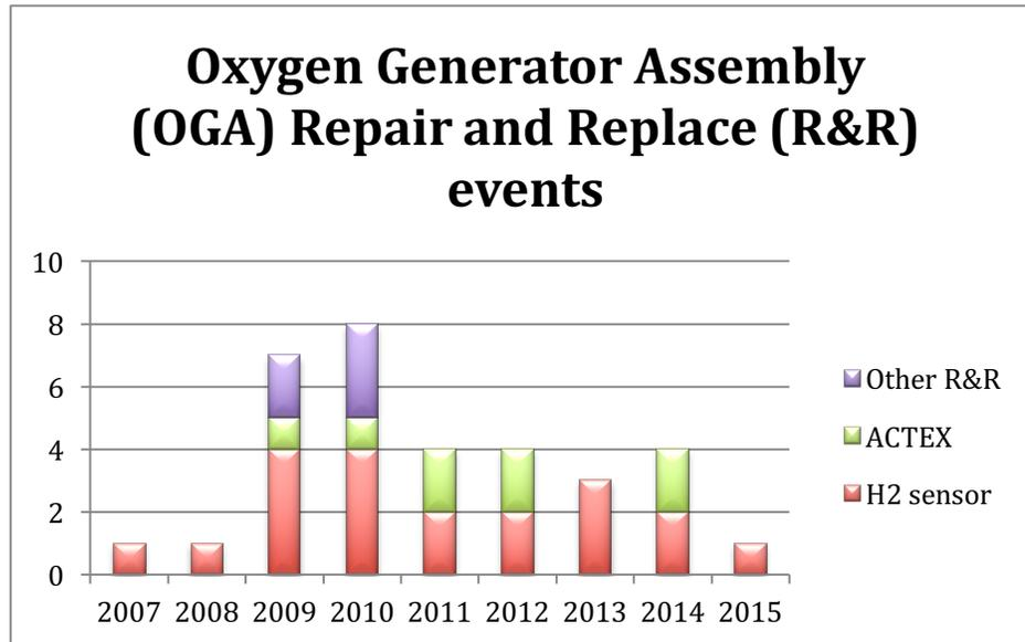
Figure 5. The number of OGA Repair and Replace (R&R) events each year for the H2 sensors, the ACTEX, and other R&R.
