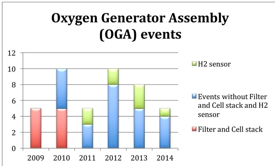
Figure 3. The number of failure and maintenance events each year without Filter and Cell stack and H2 sensor, for the combined Filter and Cell stack group, and for the H2 sensor group
