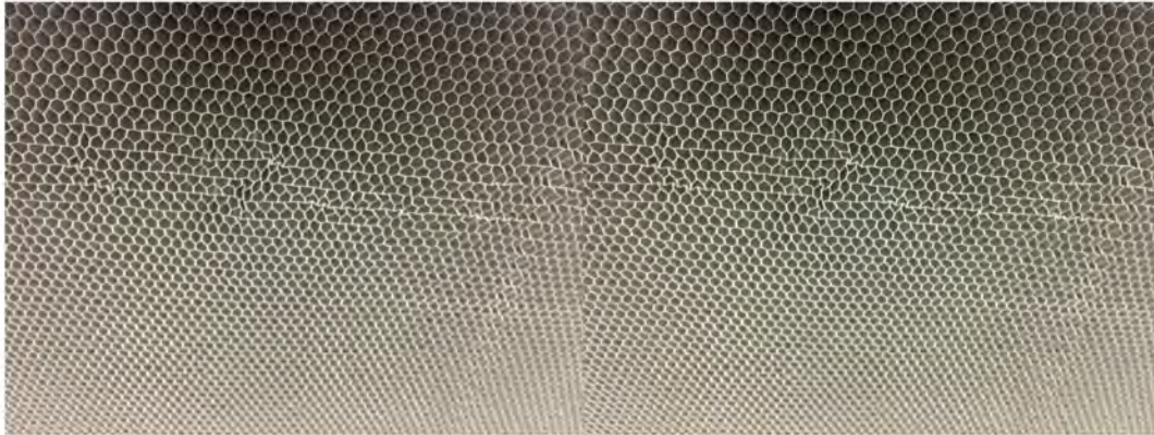
Figure 84. Honeycomb core cell irregular shapes.
