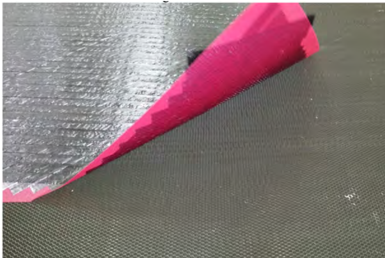
Figure 88. View of honeycomb core after fiber placement of top skin, showing no damage.
