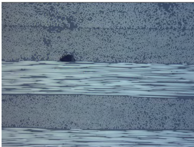
Figure 101. Example of void most likely caused from air entrapment.
