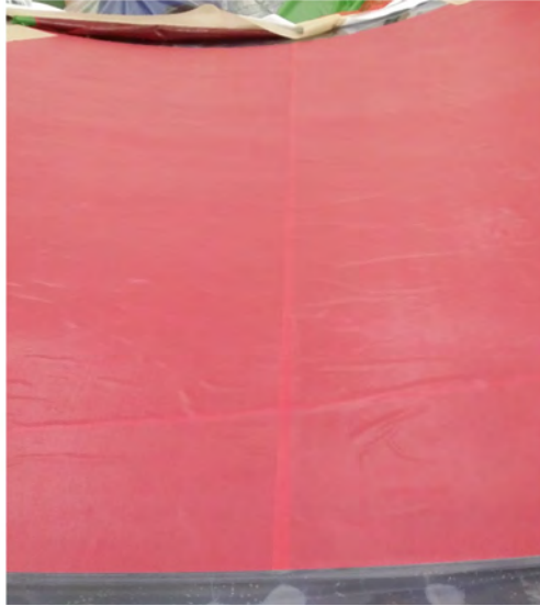
Figure 87. Second film adhesive layer with overlap.
