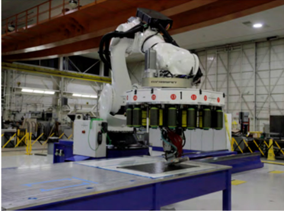
Figure 6. Equivalency panel fabrication at LaRC.
