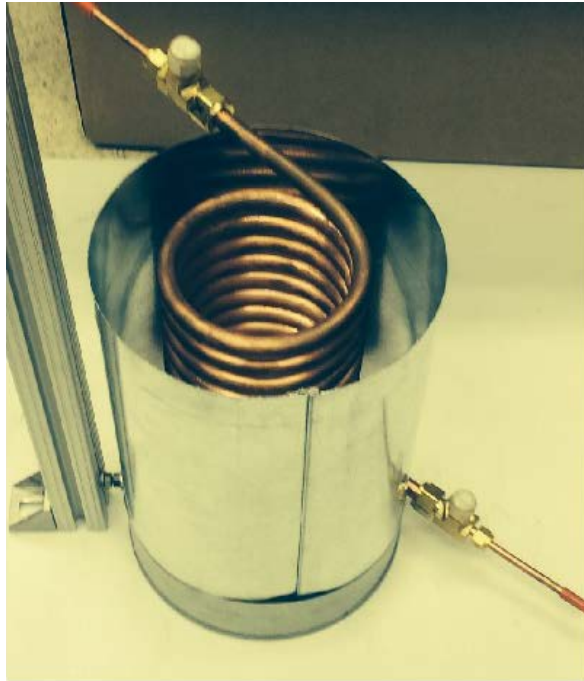
Figure 41.—Recuperative Heat Exchanger Inside.
