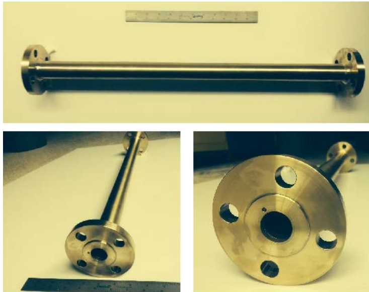
Figure 46.—Carbon Monoxide Reactor Chamber.
