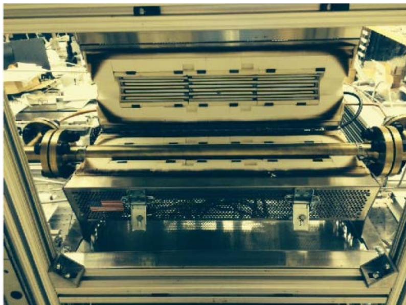
Figure 39.—Furnace Open Showing Reactor Assembly.
