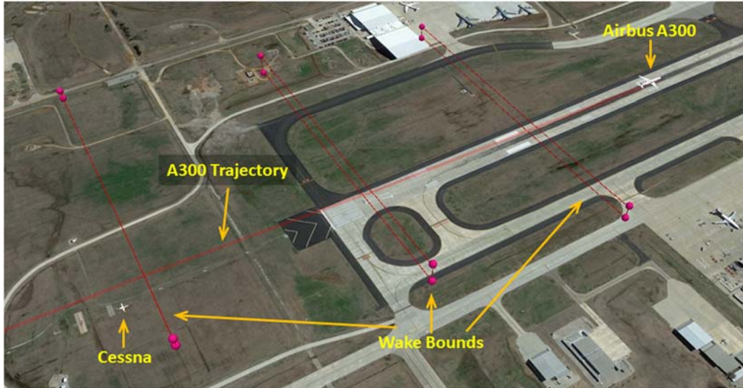
Figure 7: The A300 and its track are shown in the figure along with the APA3.4 predicted vortex bounds. The Cessna encountering the wake bounds predicted by the model is also shown in the figure (Gloude-mans et al. 2016).
