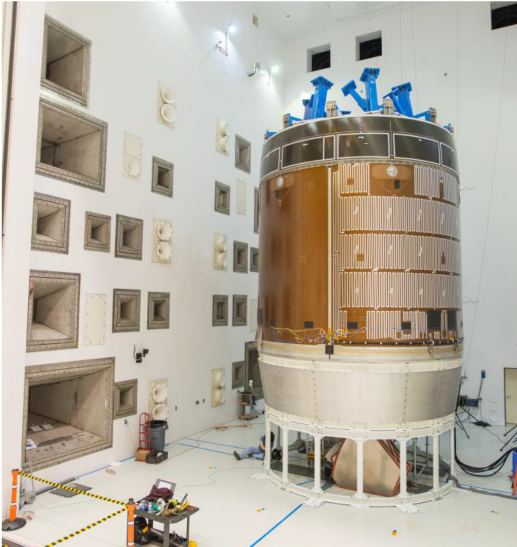
Figure 15.—E-STA with MSA simulator and test stand.
