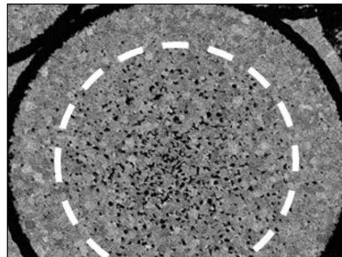
Example of Increased Amount of Porosity in SiC Fiber Core
