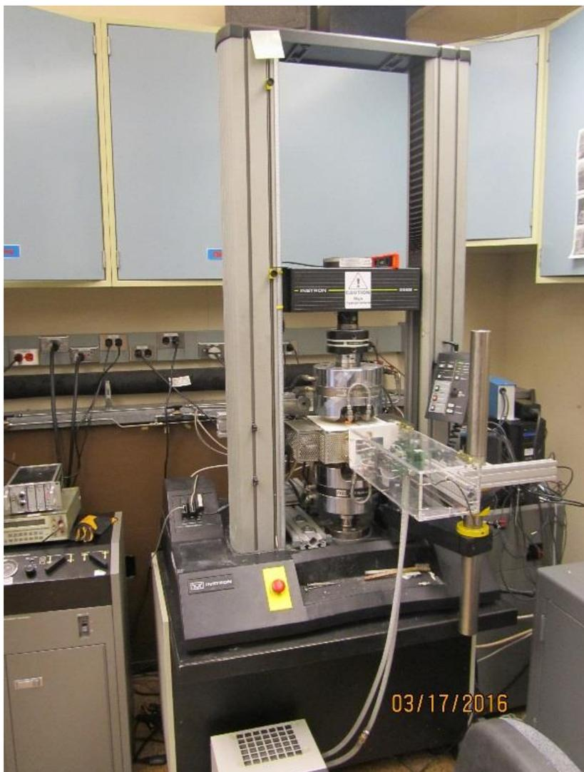
Example of Rig Used to Test SiC/SiC CMCs
