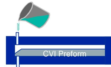
Slurry Cast SiC Particles Into Porous "Preform"
