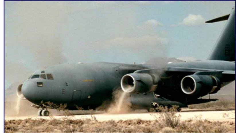
Aircraft Engines Ingesting Sand on Runway
