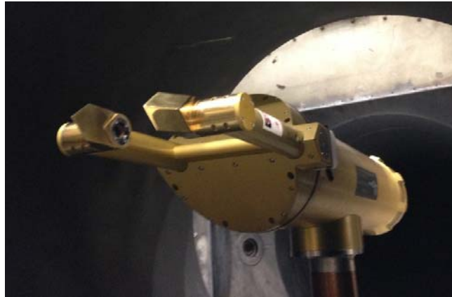
Figure 19. PSL particle sizing instruments installed at calibration plane. (a) CDP with spray on as viewed by Spraybar camera, (b) CIP.
