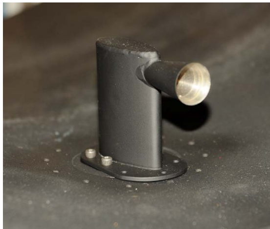
Figure 13. Reverse Flow Background Humidity Inlet.
