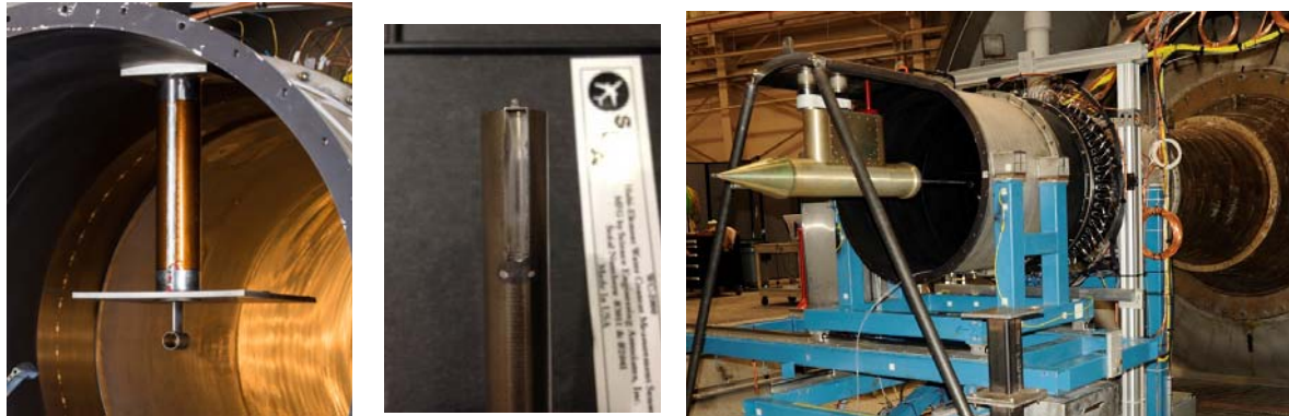
Figure 10. TWC sensors: (a) Multi-wire installed in PSL, (b) Robust Probe and (c) IKP2.
