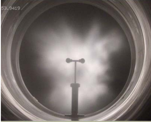
Figure 19. PSL particle sizing instruments installed at calibration plane. (a) CDP with spray on as viewed by Spraybar camera, (b) CIP.
