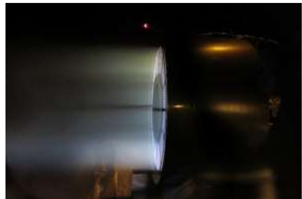
Figure 2. Full-Scale GEN2 AIE in Test; 65 cm outside Beam Diameter
