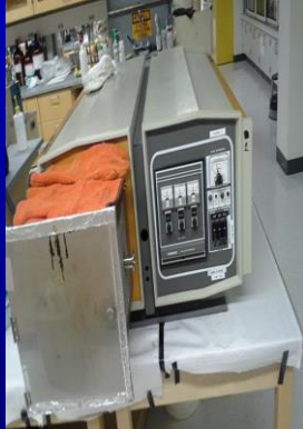
Three zone CVD growth furnace
