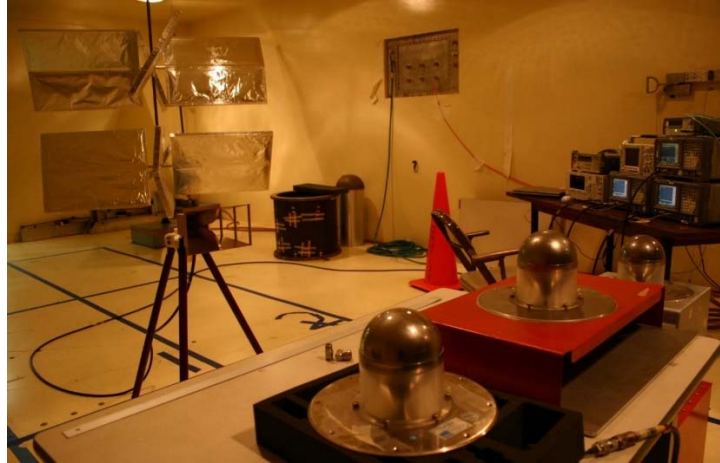
Figure 24. Test setup inside the reverberation chamber with the transmit antenna pointing directly at three D-dot sensors that acted as the receive antennas. All three receive antennas were used for the antenna diversity study while only one was used for the frequency diversity study
