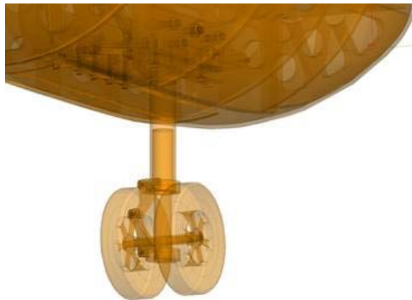
Figure 3. CAD model of the nose landing gear of the GMA-TT UAV used for the computational modeling task of EWAIC
