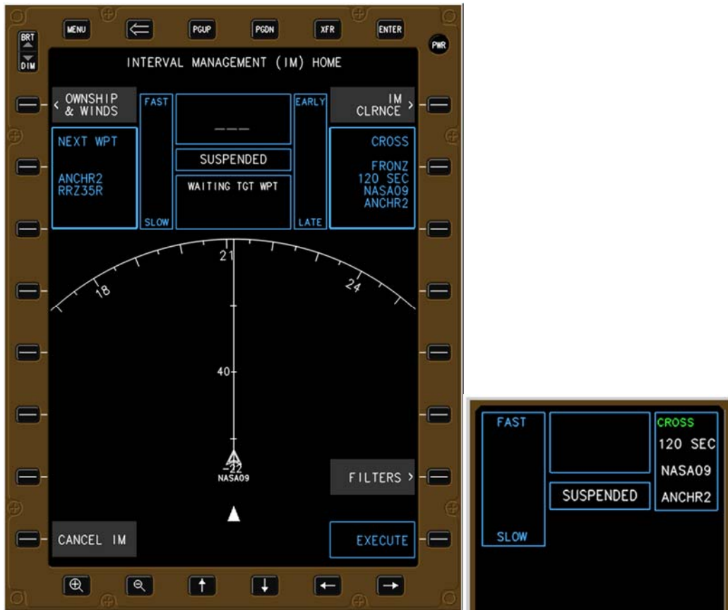
Figure 60. EFB and CGD in the SUSPENDED-ARMED state.
