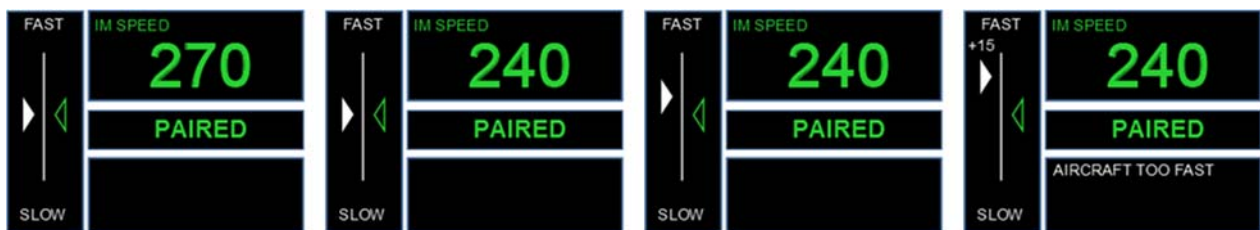
Figure 63. FAST/SLOW indicator sequence during IM speed change.
