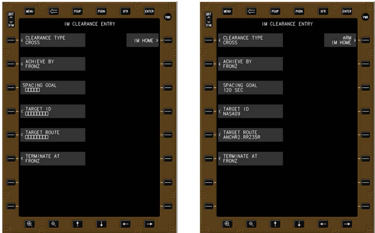
Figure 72. IM CROSS clearance page with and without data entered.
