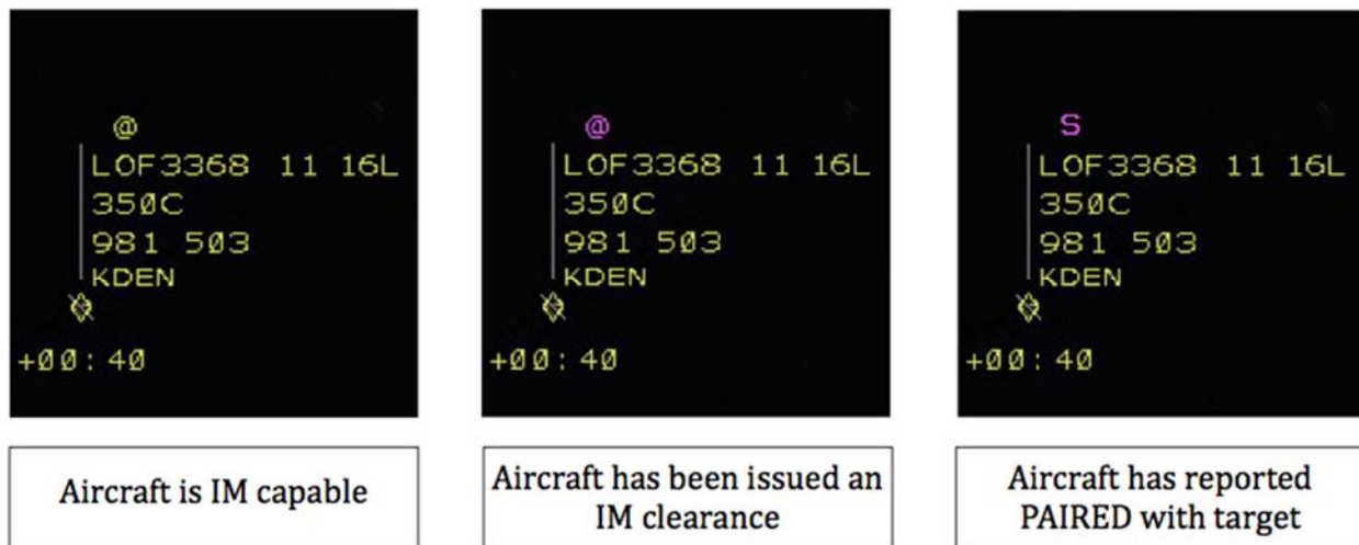
Figure 4. IM status indications on the ARTCC controller workstations.
