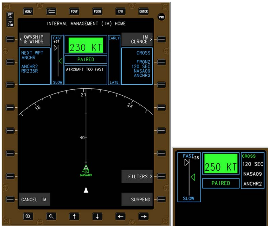
Figure 62. EFB and CGD with IM speed in reverse video.
