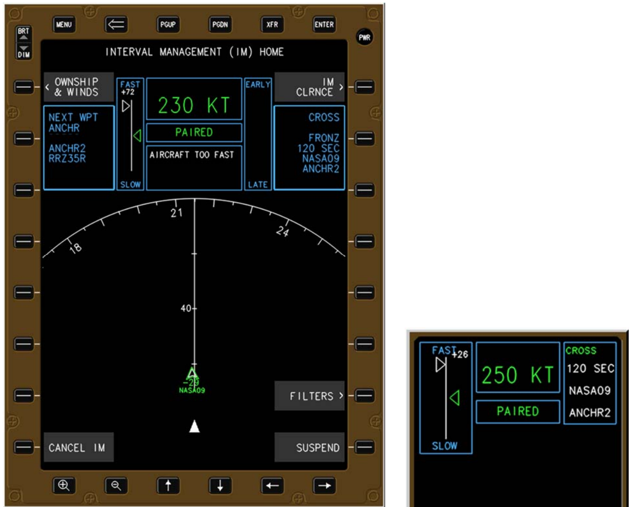
Figure 6. IM Cockpit Interfaces: EFB (left) and CGD (right).
