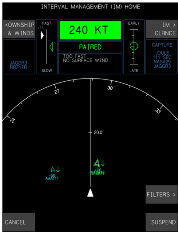
Figure 77. PAIRED and SUSPENDED-AVAILABLE states in the DTS and IFD.
