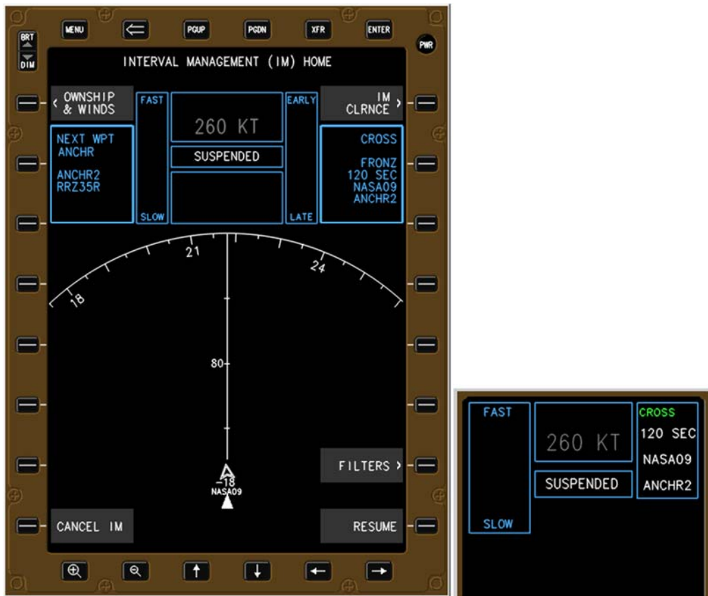
Figure 59. EFB and CGD in the SUSPENDED-AVAILABLE state.
