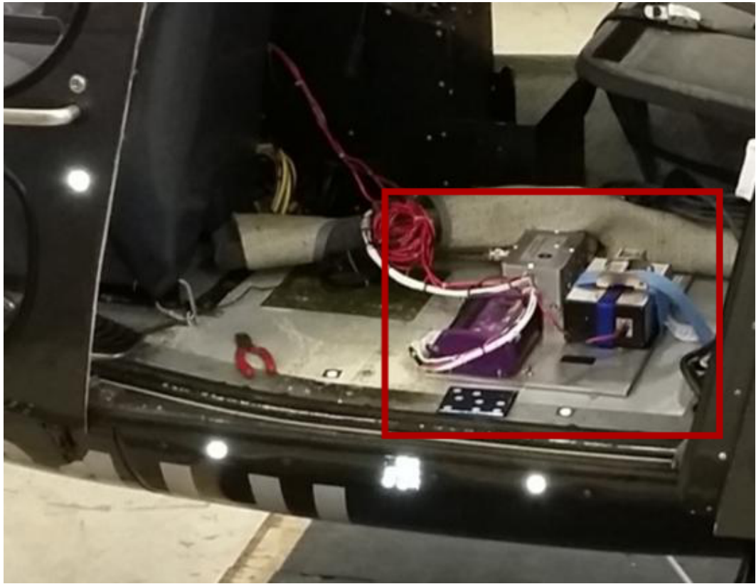
Figure 9: Instrumentation pallet installed in AS350 SD1.
