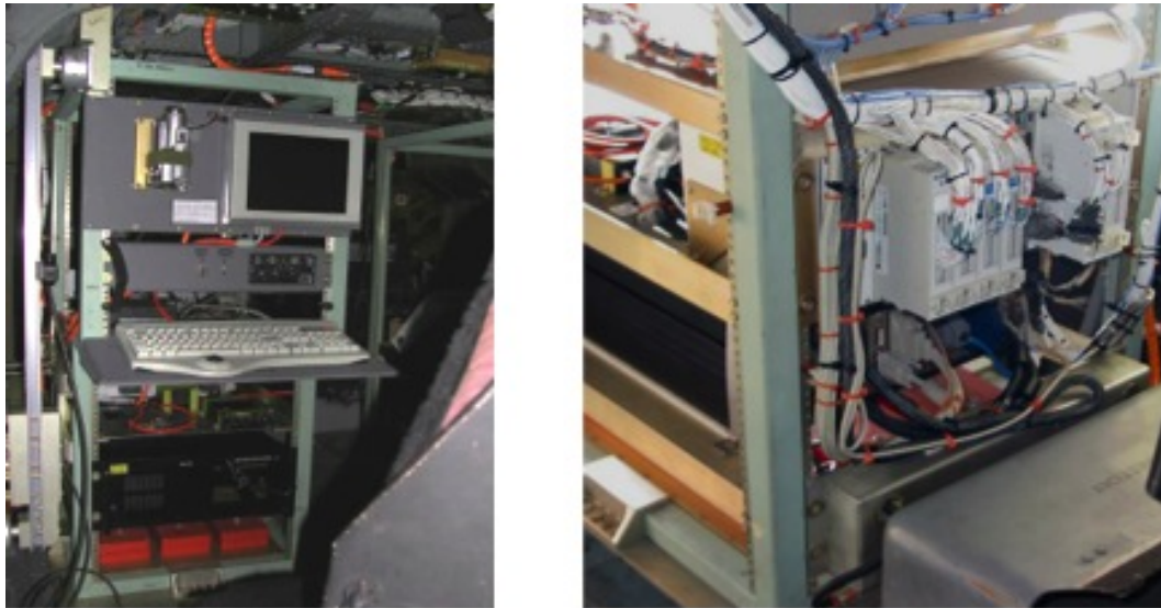
Figure 11: EH-60L Aircraft Data System computer and signal conditioner.
