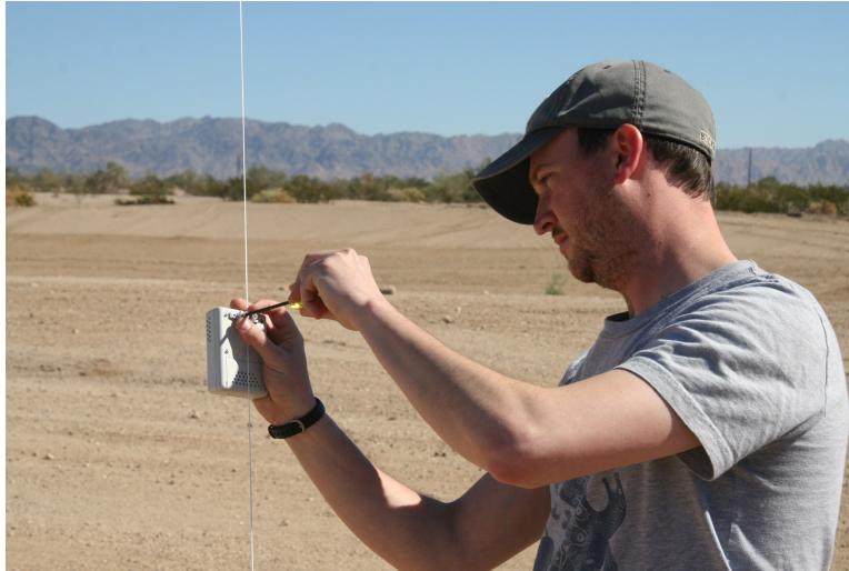
Figure 19: Temperature sensors being mounted on balloon tether.
