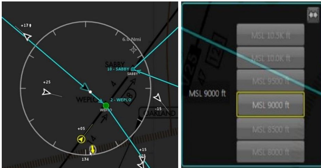
Figure 1. Vector planner horizontal and vertical guidance displays
