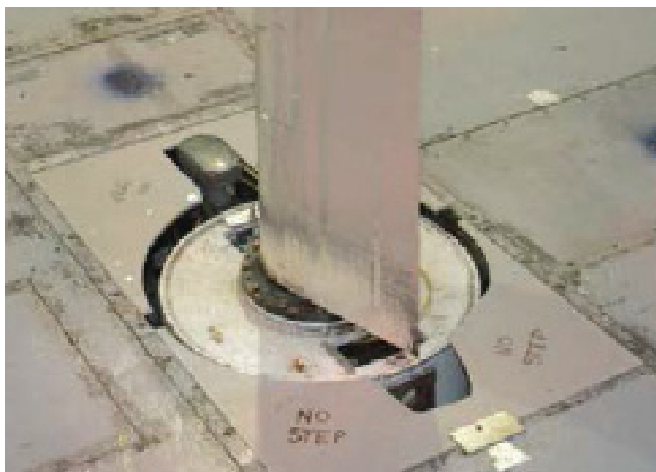
Figure 17: Picture of the floor cavities beside the test stand in the 7- by 10-foot wind tunnel [3].
