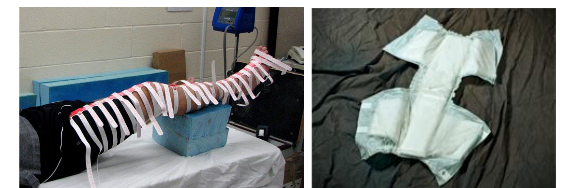
Figure 5. Circumferential measurements of the leg used in the construction of the custom-fitted GCG (left). Example of MAG (right) worn by astronauts under the space suit for collection of urine and feces.
