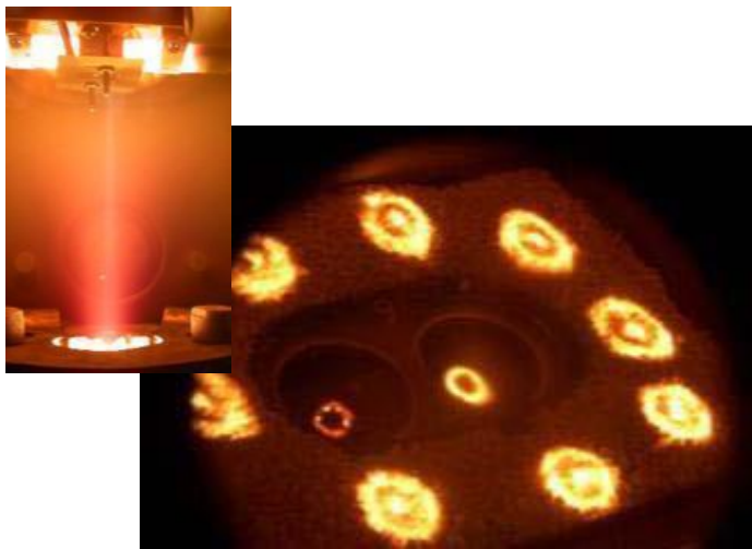
Triplex Pro (Oerlikon Metco) Processing and Advanced NASA EBCs – combustor liner demos
