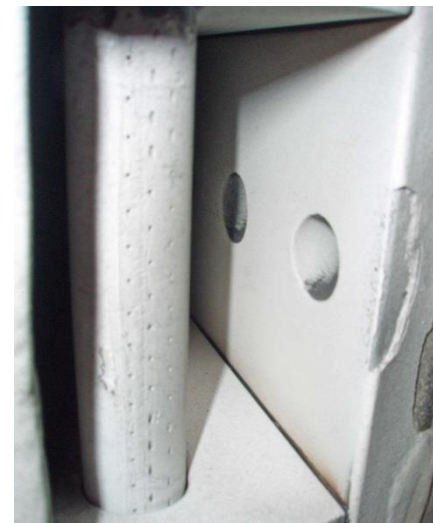
EBC Coated Prepreg SiC/SiC vane tested 75 hour testing at 2650°F
