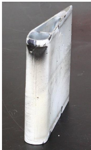
EBC Coated Prepreg SiC/SiC vane after 21 hour testing at 2500°F
