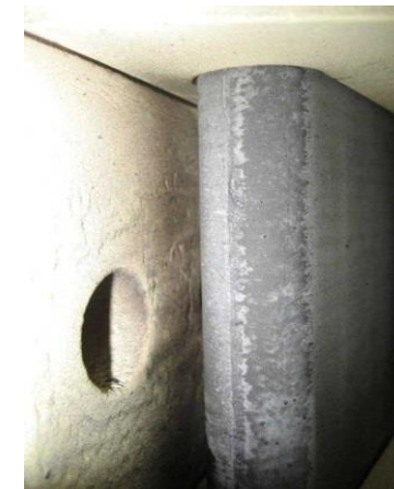
Uncoated vane tested 15 hr
