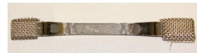
PVD GdYbYSi coated on GE Prepreg SiC/SiC 1316°C, 15ksi, 1169 h fatigue (3 Hz, R=0.05)
