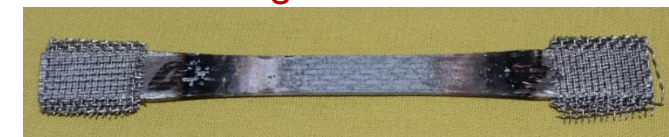
PVD GdYSi coated on Hyper Them CVI-MI SiC/SiC 1316°C, 10ksi, 1000 h fatigue (3 Hz, R=0.05)
