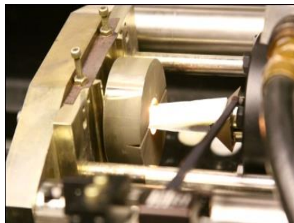
Advanced EBC coated CMC subelement testing and modeling
