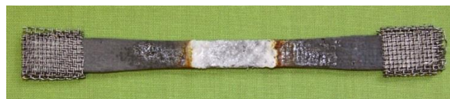
Air Plasma Sprayed YSi+Hf-RESilicate EBC Bond Coat series on CVI-MI SiC/SiC 1400°C, at 10 ksi, 400 hr
