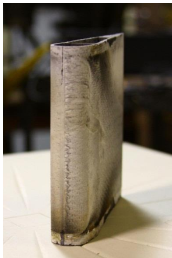
EBC Coated CVI SiC/SiC vane after 31 hour testing at 2500°F+ coating temperature
