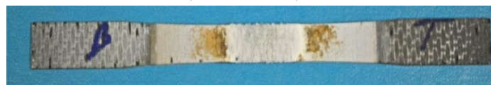
EB-PVD (Hf, Yb, Gd, Yb)_2Si_{2-x}O_{7-x} EBC/GdYbSi bond coat on Rolls Royce CVI-MI SiC/SiC (with CMAS) 1537°C, 10ksi, 300 h fatigue (3 Hz, R=0.05)
