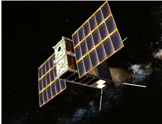
Figure 4: Proposed SPAGHETI 6U deep-space CubeSat
