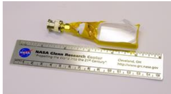
Figure 8: Miniature scintillation/diode ionizing radiation detector as demonstrated
