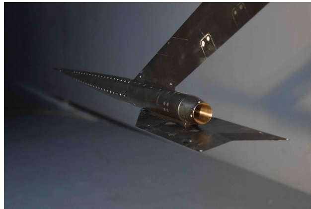
Figure 16. The Aft deck shield model installed in the test section.
