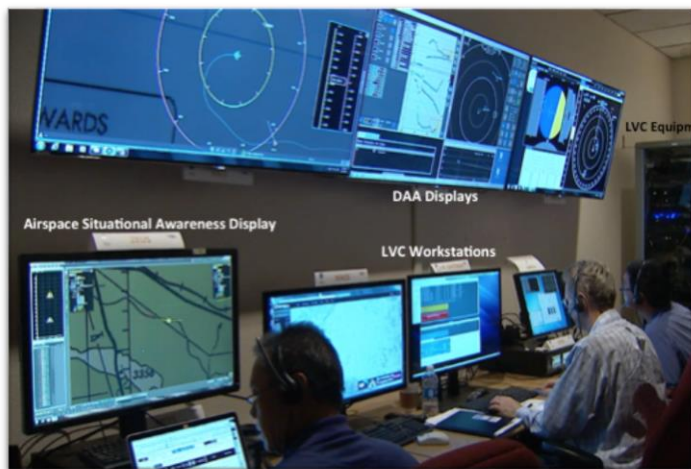
AFRC: Display replication for video streaming to support UAS flight test remote monitoring
