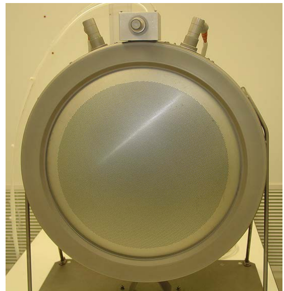
Figure 1. Pretest image of the NEXT LDT thruster.
