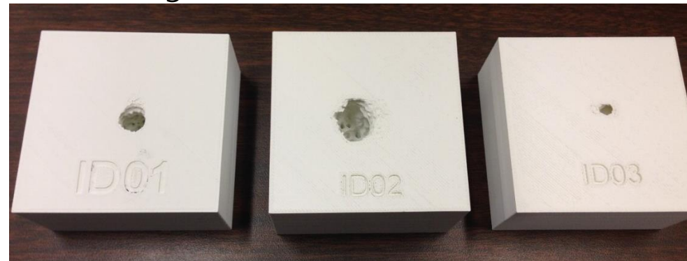
Example Prints from a Stratasys Fortus 400mc Slice height of .005" Model Material - ASA
