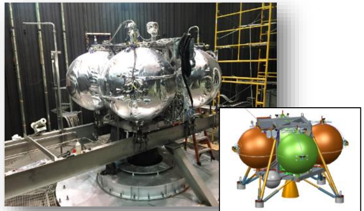
Figure 1: Integrated Cryogenic Propulsion Test Article (ICPTA) installed in the NASA Plum Brook In-Space
