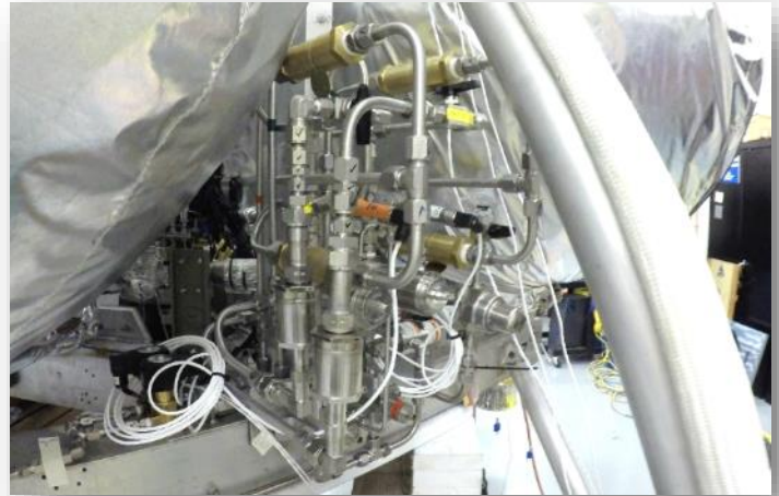
Figure 2. ICPTA Helium Regulation and Control Panel
