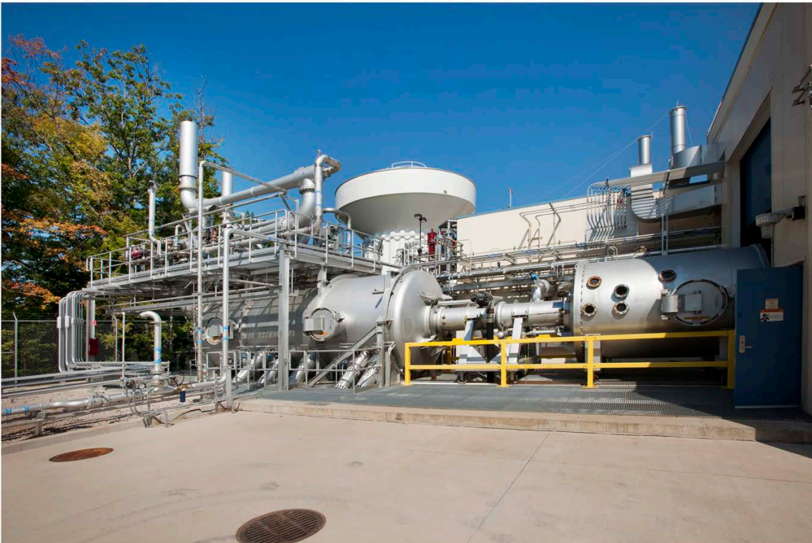
Figure 4: Exterior photo of the Altitude Combustion Stand's translating test chamber, water cooled diffuser, spray cooling condenser, and vacuum ejector systems.
