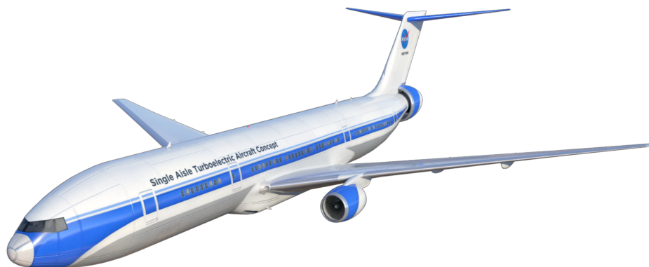
Figure 1: NASA's Starc-ABL aircraft concept, incorporating a hybrid electric propulsion system and aft-mounted BLI propulsor [4]
