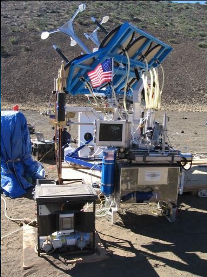
Carbothermal Regolith Reduction Module, Solar Energy Module and Pneumatic Regolith Transfer Unit during the 2010 ISRU Analog Test.
