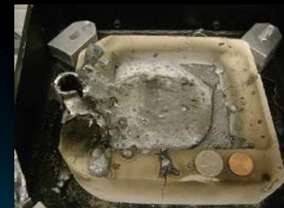
Small casting of molten ferrosilicon (lower layer) and molten oxide of lunar composition (top layer) withdrawn by counter-gravity suction at 1600C from reactor furnace (Image credit: Ohio State U./KSC)
