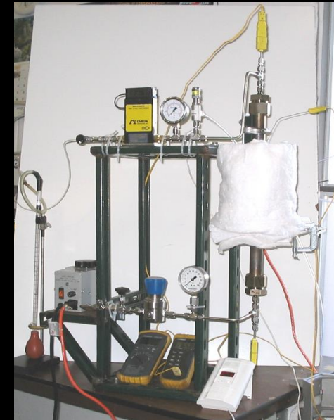
Iron Oxide Reduction - Carbon Deposition Reactor (81 g JSC-1)
