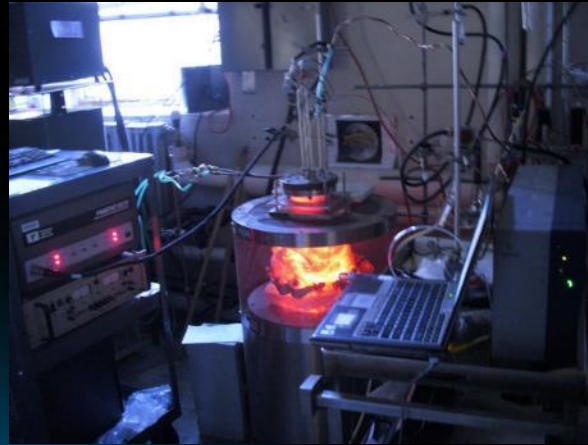
Schematic of electrolytic cell configuration to investigate electrochemical behaviors of various anode materials in molten oxides (left) and furnace containing the cell in operation at 1600°C (right) (MIT)
