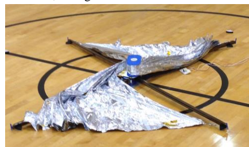
Fig. 7. Demonstration of sail unspooling during deployment
