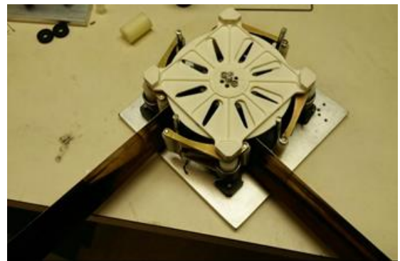
Fig. 2. Early Prototype of TRAC boom deployer, single spool
