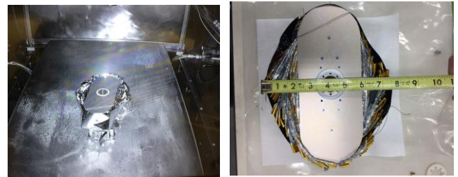
Fig. 9. Sail spool during ascent vent testing (left) and post evaluation (right)
