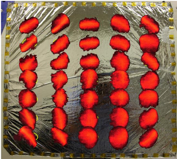
Figure 3) Test Material Showing Shape of Reflected Light Pattern with Grid at 2, 3, 4, 6, 8, 10 and 12 Degrees
