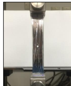
Fig. 4. Setup for tensile test of metallized PEN film with a 2 mm die-cut hole to simulate potential impact damage.
