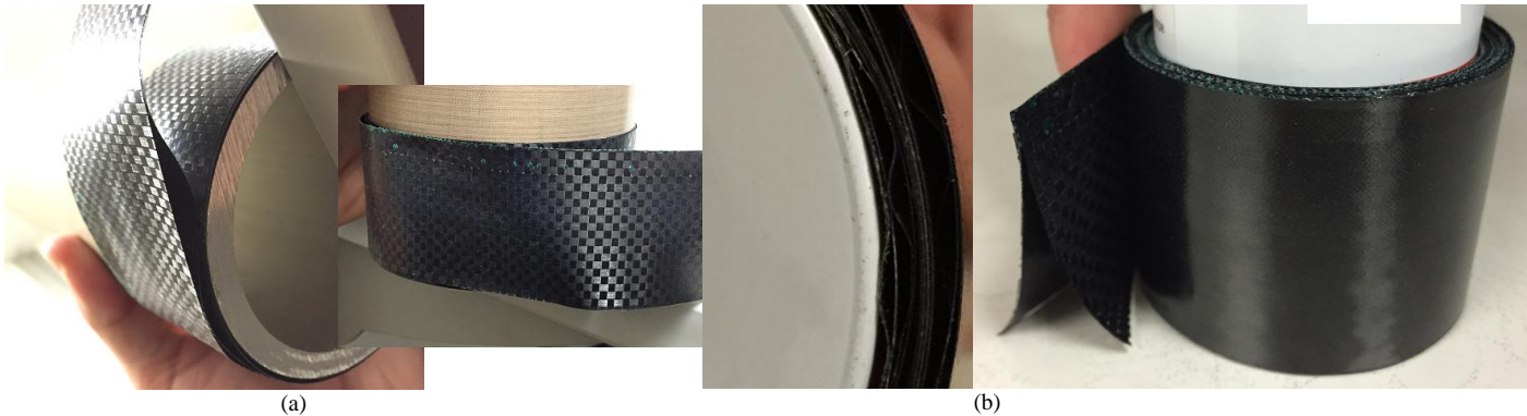
Fig. 8. (a) Inner shell bifurcation causing global deformation for the v7 laminate; (b) inner shell local buckling contained within the coil for the v6 laminate. The outer diameter of the coil measured at the web and flanges sections are very similar, which indicates a small loss of packaging efficiency.
