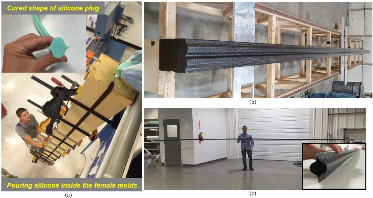
Fig. 5. (a) Silicone plug mold fabrication process and final shape; (b) two-part 7.3 m carbon mold axially aligned and assembled; (c) 7 m long mini-CTM / omega boom self-supporting under gravity with a close view of its cross-section.
