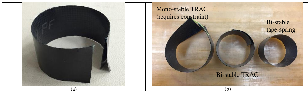
Fig. 9. (a) Bi-TRAC_v16 in a stable coiled state; (b) Comparison between bi-stable and mono-stable coiled booms. The Bi-TRAC coiled behavior is similar to that of standard bi-stable tape-spring.
