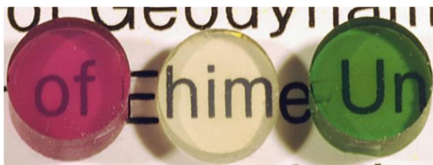
Figure 2. High-quality polycrystalline garnet synthesized at 15 GPa and at 1,400 °C, with a diameter of ~4 mm and thickness of ~2 mm; grossular with 2 mol% \text{Ca}_3\text{Cr}_2\text{Si}_3\text{O}_{12} uvarovite (green), pure grossular (colorless, hardness of ~14Hk) and \text{Mg}_3\text{Al}_2\text{Si}_3\text{O}_{12} pyrope with 5 mol% knorringite \text{Mg}_3\text{Cr}_2\text{Si}_3\text{O}_{12} (purple). After [3].
