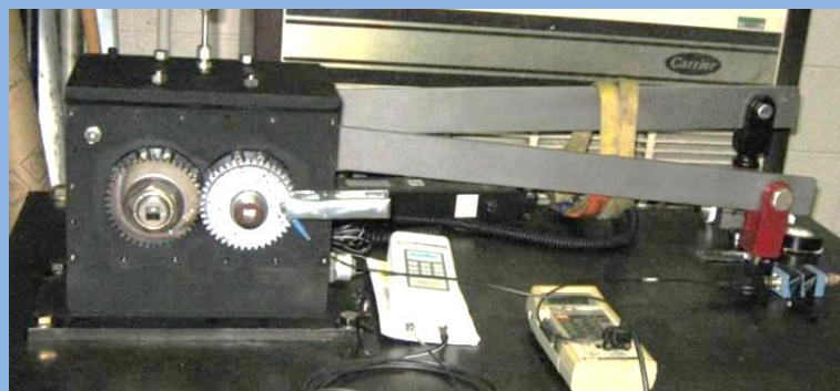
Static torque tests on coupon level gears
