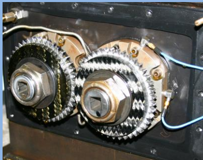
Endurance testing of 3.5" pitch diameter coupon gears
