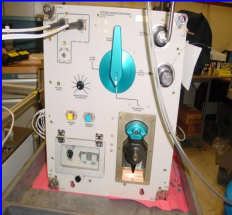
Potable Water Dispenser
