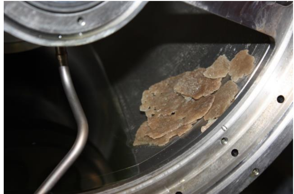
Calcium sulfate precipitation in the Urine Processor Assembly (UPA)
