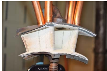
Cr:GAP coated vane with cooling air supply tubing
