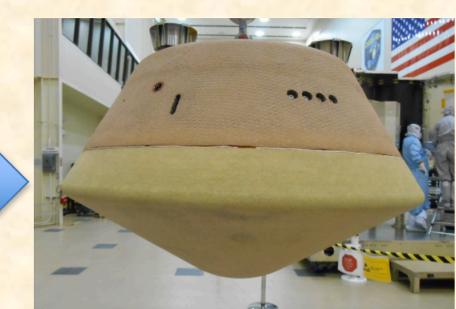
Single piece PICA heatshield (< 1.25m max diameter)
