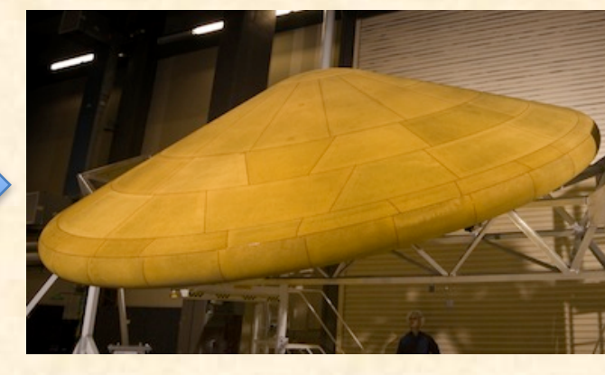
Tiled PICA heat shield (> 1.25m max diameter)
