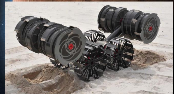
RASSOR (Regolith Advanced Surface Systems Operations Robot) will feed the hopper (2 x 40 kg drums, 25 cm/s, 60% on duty time)
