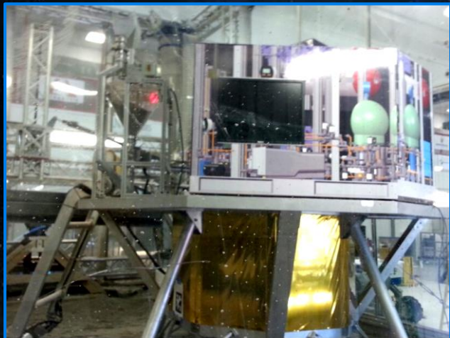
KSC: Mockup Lander w/Hopper, Mock Oven, and APM Simulator in Regolith Bin
