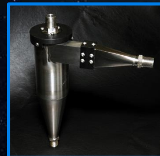
Cyclone separator prototype. 10" tall, 2.4" inner diameter. Smaller prototypes were built.
