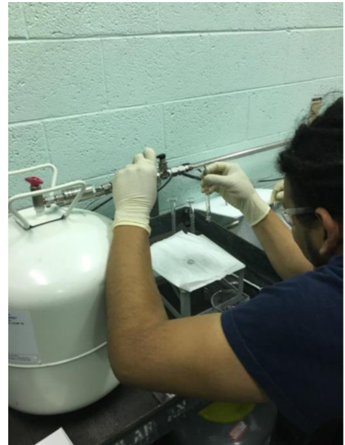
Filtered solvent is dispensed directly from the cylinder into a syringe equipped with a gas tight valve at the outlet.
