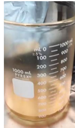
Contaminated Big Red / Solstice Spray effluent
