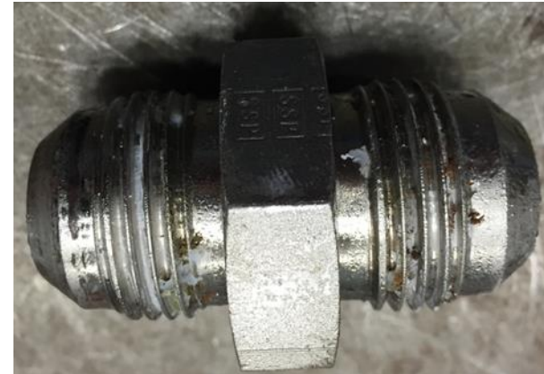
LOX Fitting with Contamination
