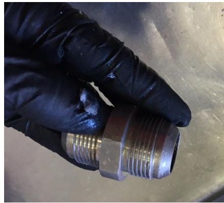
LOX fitting post Solstice PF Spray Clean
