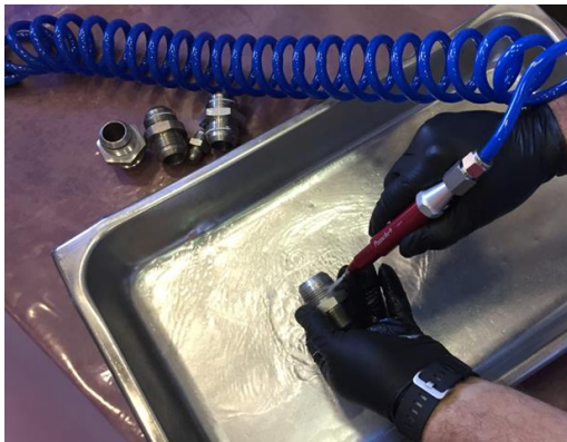
Solstice PF Spray Cleaning of LOX Fittings
