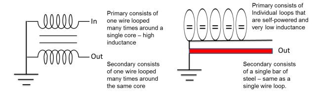
Each 'Pie-Slice' provides a simultaneous parallel pulse to the inductor For increased current (and thus B-Field)
