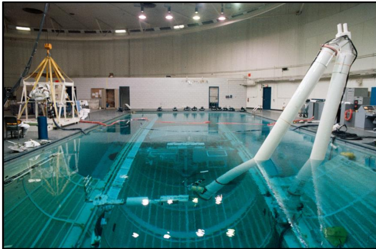
Figure 3. The Weightless Environment Training Facility (WETF) with the Space Shuttle cargo bay and robotic arm submerged in the pool (photo courtesy of NASA).
