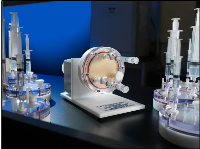
Figure 1. Rotating wall vessel (RWV) developed by NASA and used during ground-based microbiology experiments. Image: NASA
