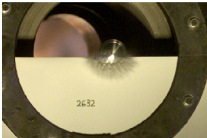
Fig. 42. Four frames from a high speed video showing a LDS model penetrating the slap paper.
