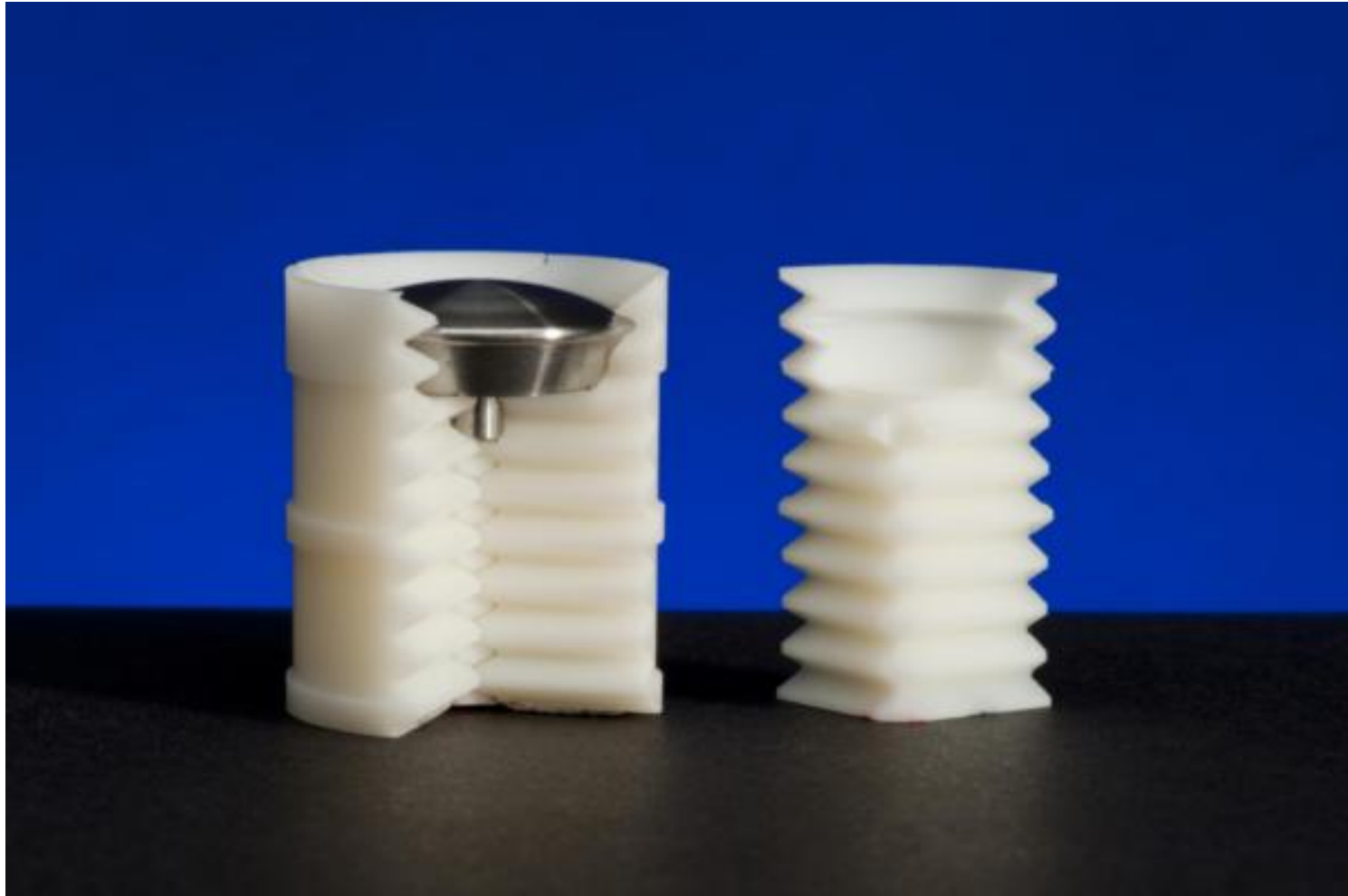
Fig. 2. Model inside 3 of 4 serrated sabot fingers. Fourth sabot finger is off to the right.
