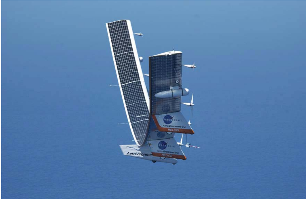
Figure 1. A super-long flying wing Helios prototype (wing span 247 ft) under very high wing dihedral deformation just before breaking up.
