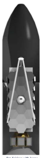
8m fairing with large aperture telescope
